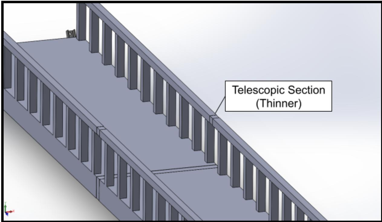
As the angle changes, the slope will adjust but retain an ADA-compliant slope of 1:12. The changes made to the ramp do not add barriers or add any difficulty for people with disabilities. The ramp is easily accessible and does not interfere with their ability to get to the riverboat.
