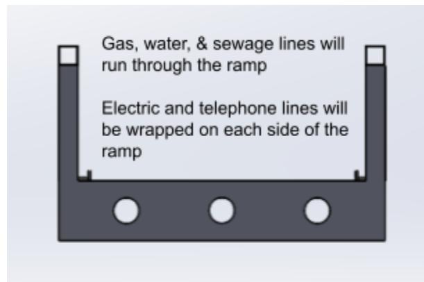
The electric and telephone lines will be looped around the telescopic section of the ramp so if the ramp expands, the utility lines will be able to unravel and maintain their constant tension.
