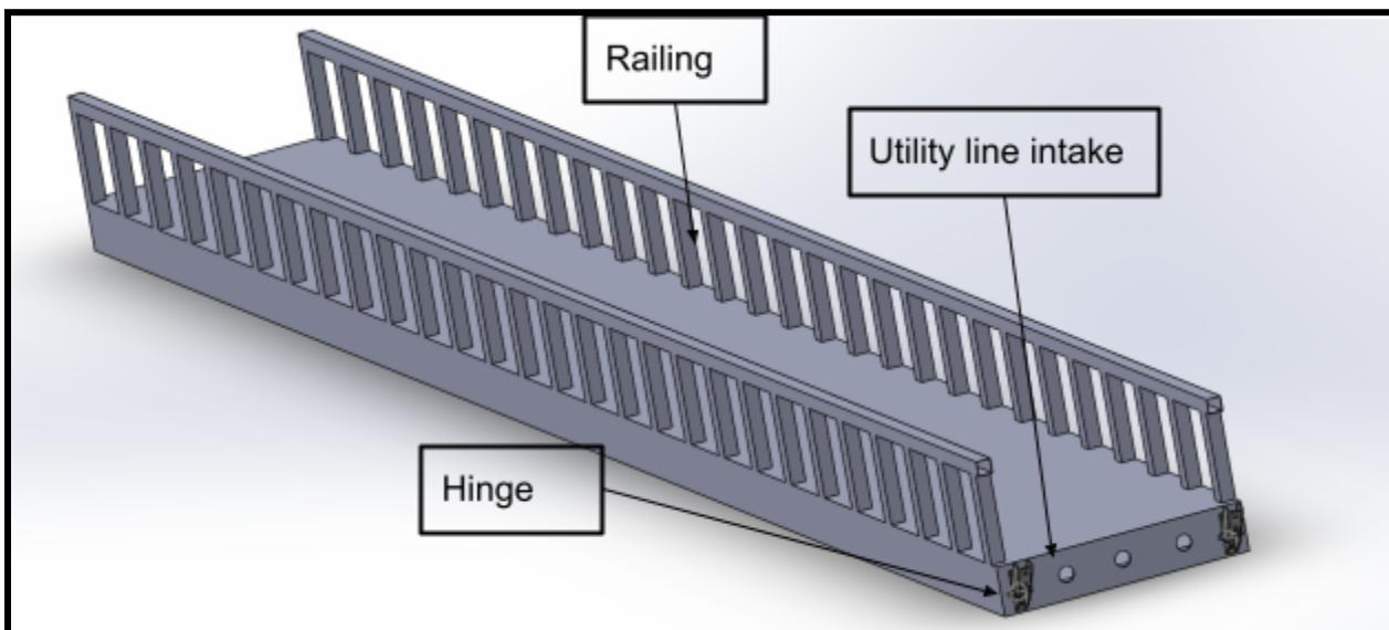
The last major change we will be making with the bridge is we are making the bridge telescopic allowing it to extend without having the dock move. The section of the railing that will be telescopic will just be a little bit that accordions. The section of the bridge that is telescopic will have a skinner part inside it that is able to move in and out.
